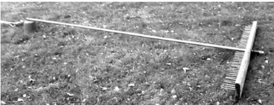
Rick's home-made milfoil rake. More specific instructions for building this tool are available on our website www.IndianRiverLakes.org .
